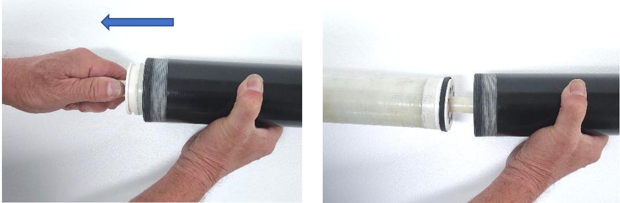
Figure 32: Pulling the Membrane Element Out
