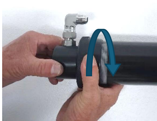
2. Thread the Ring on until the End Cap Seal contacts the Tube
