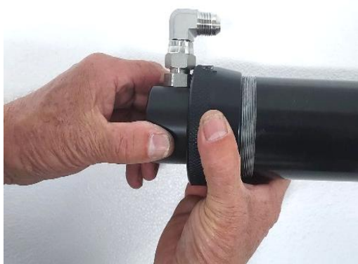
3. Twist and push the End Cap until the Seal goes in the Tube
