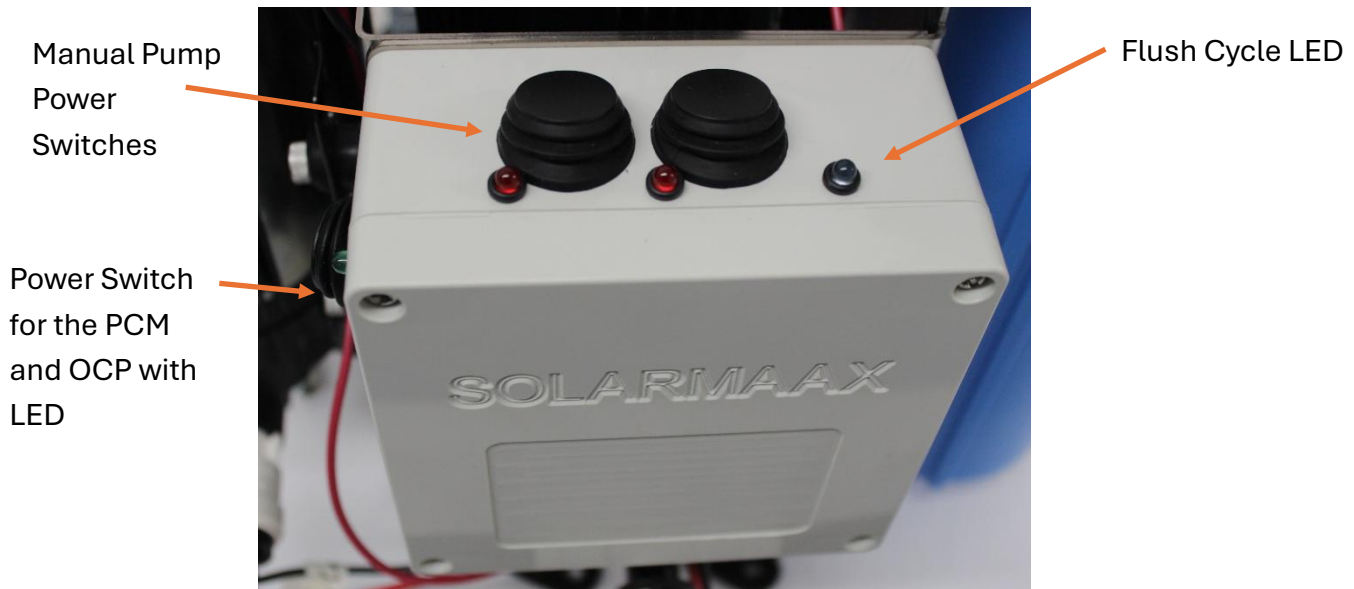
Figure 25: Pump Control Module (PCM)
